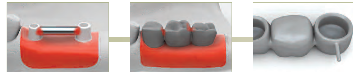
Fabricate burn-out cylinder and plastic bar in preparation for wax-up
